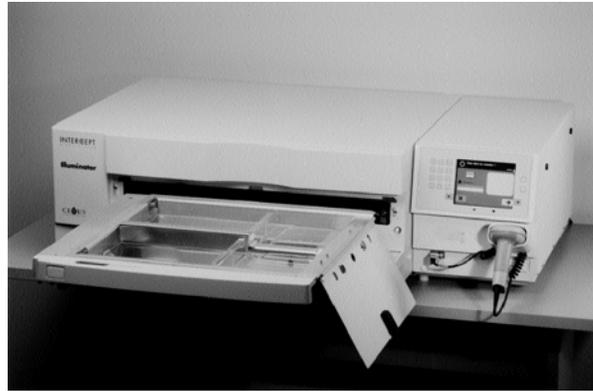
One blood product and processing set fits in the front chamber, chamber 1. The blood product in the illumination container goes on the left side of the chamber, with the rest of the set on the right side of the chamber.
