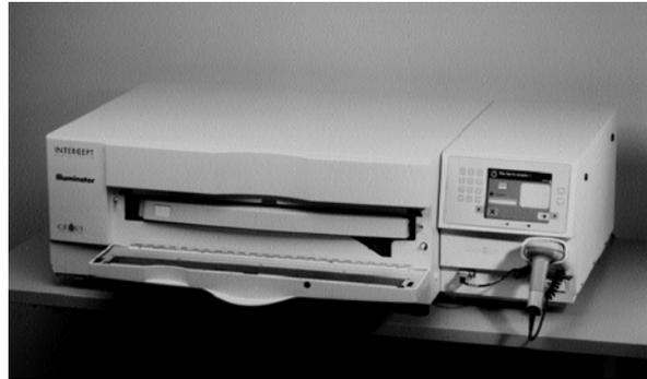
Inside, a drawer pulls out. The clear tray where illumination is performed is held in the drawer. The drawer is on a flatbed agitator, so that blood products are agitated when they are in the illuminator. There are four compartments in the tray to hold blood products and the accompanying processing sets during illumination.
