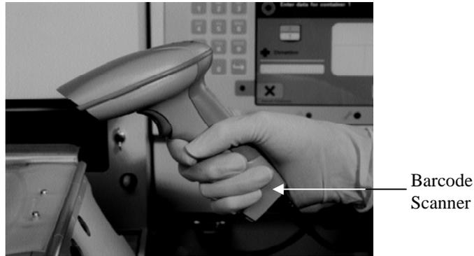
Barcodes are used to track blood products through the INTERCEPT Blood System process and can be found on the final storage container label of the INTERCEPT Processing Set.
