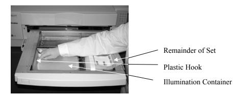
10. Put the tubing from the illumination container in the slot of the divider. Make sure that the sealed tubing containing blood product is within the left-hand side of the chamber.
