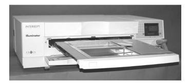
There is a cover for the two compartments on the right side, designed to keep the set and tubing from getting caught during agitation. The operator opens this cover to load the set and closes it before beginning illumination.
